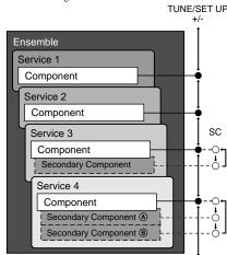
When the selected secondary component is finished, the unit returns automatically to the former primary
